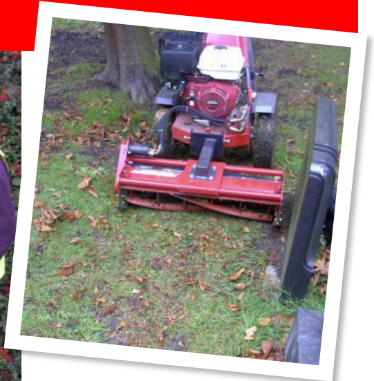
Above: KCM976 mowing deck cuts close to obstacles reducing the need for secondary mowing.
